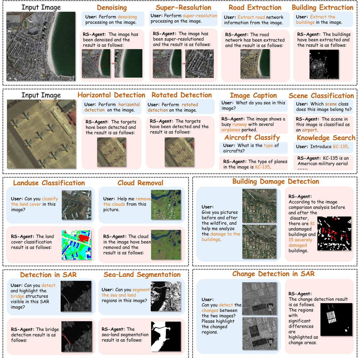
Figure 4 (Color online) Qualitative result of RS-Agent. This figure shows several key tools that highlight the core capabilities of RS-Agent. The input image represents the image input by the user. The blue box shows the user's request, and the red box shows the RS-Agent's reply.
