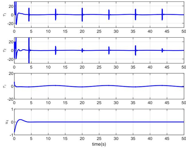
Figure H9 The control inputs under circle-shape trajectory tracking.
