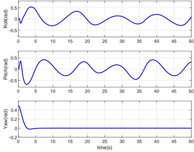
Figure H8 Attitude angles under circle-shape trajectory tracking.
