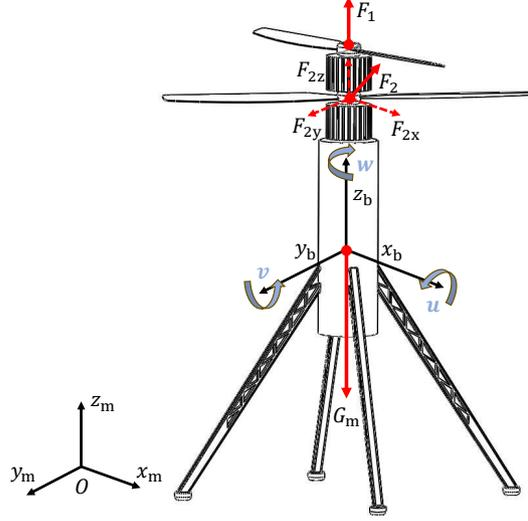
Figure A1 Configuration of the Mars coaxial rotors UAV.
