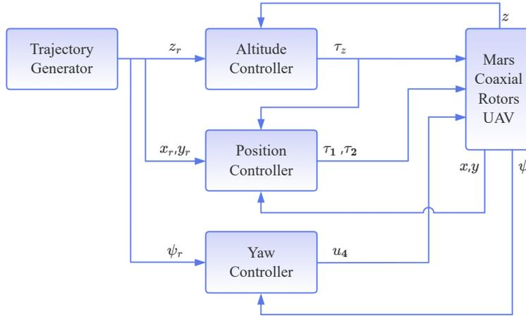
Figure B1 Block diagram of the control system.
