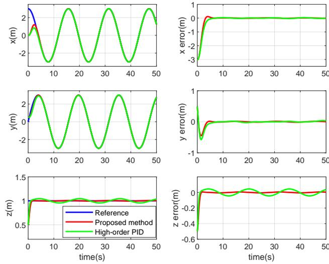
**Figure H7** Circle-shape trajectory tracking results in three directions.
