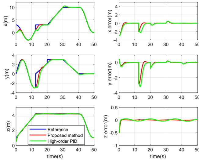
Figure H3 Trajectory tracking results in three directions.
