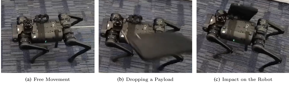
Figure A5 A solid payload that weighs about 3kg is dropped from the air on the top of the robot during walking.
