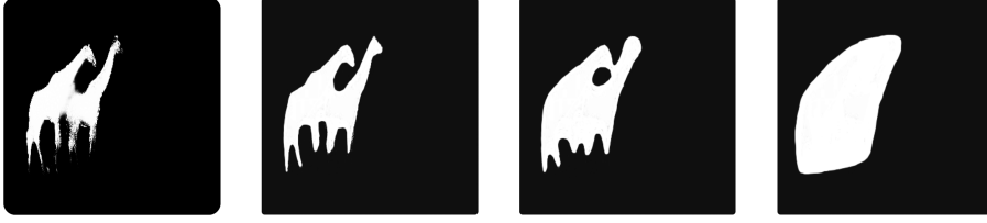
Figure 6 Examples of gradual dilation of the foreground mask. The larger the dilation effect, the less information about the foreground class is contained in the saliency map.
