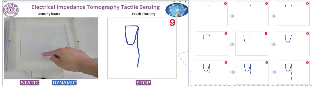
Figure D5 Schematic diagram of touch tracking based on the proposed sensor.
