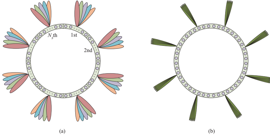
Figure 4 (Color online) Illustration of the designed hierarchical codebook. (a) The first layer; (b) the second layer.
