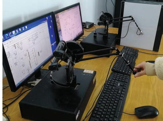
**Figure 9** (Color online) Experimental platform of networked teleoperation systems.
