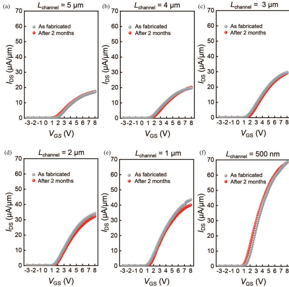
**Figure 5** (Color online) Transfer characteristics of MoS<sub>2</sub> FETs with Bi/Sb/Au contact electrodes with different  $L_{\text{channel}}$  as fabricated and after two months, including (a)  $L_{\text{channel}} = 5 \mu\text{m}$ , (b)  $4 \mu\text{m}$ , (c)  $3 \mu\text{m}$ , (d)  $2 \mu\text{m}$ , (e)  $1 \mu\text{m}$ , and (f)  $500 \text{ nm}$ .
