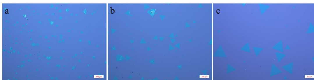
Figure S1. The low to high magnification of optical images of obtained bilayer WS 2 sheets with the assisted of carbon. (a) Low magnification of optical images of obtained bilayer WS 2 . (b) Higher magnification of optical images of obtained bilayer WS 2 . (c) High magnification of optical images of obtained bilayer WS 2 .
