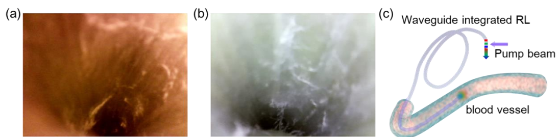
Figure S10. Image of inner wall of scallion leaf taken under (a) the waveguide integrated RL and (b) the commercial endoscope. (c) Schematic illustration of the fiber-integrated RGB RLs as an optional source for high resolution imaging.
