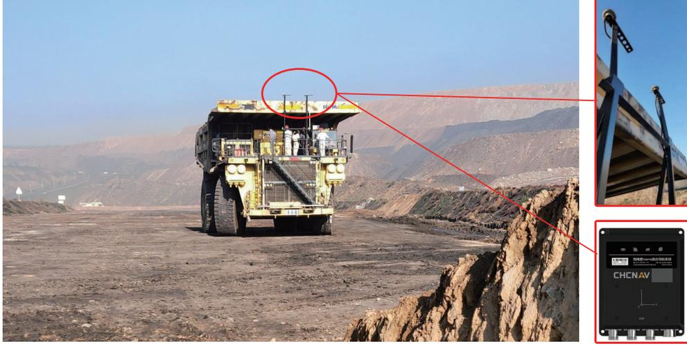
**Figure 2** (Color online) AHMDT platform used in the experiment.
