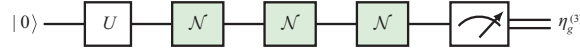
Figure 2 (Color online) Experimental setup for estimating E_g^{(3)} , where the noisy gate device (box in green) is executed 3 times sequentially.
