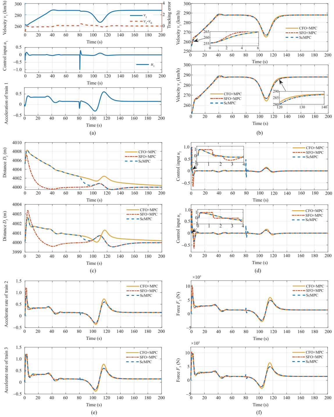
Figure 3 (Color online) States of trains under three kinds of cost functions. (a) Velocity, acceleration, and control input of train 1; (b) velocity of train 2 and train 3; (c) tracking distance of train 2 and train 3; (d) control input of train 2 and train 3; (e) acceleration of train 2 and train 3; (f) traction/braking force of train 2 and train 3.
