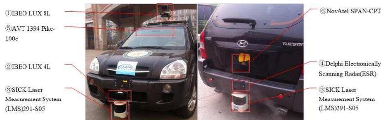
Figure A2 Mengshi intelligent vehicle sensor mounting position.
