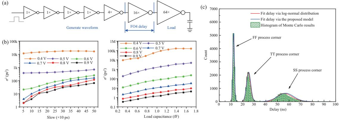
**Figure 1** (Color online) (a) Schematic of an FO4 inverter; (b) the impact of input slew and output load on  $\sigma^2$ ; (c) simulation and predicted  $\sigma_{\text{path}}$  and  $\mu_{\text{path}}$  by the proposed model or log-normal distribution at TSMC 28 nm, SS/TT/FF corner, 0.3 V, 25°C (10k Monte Carlo).
