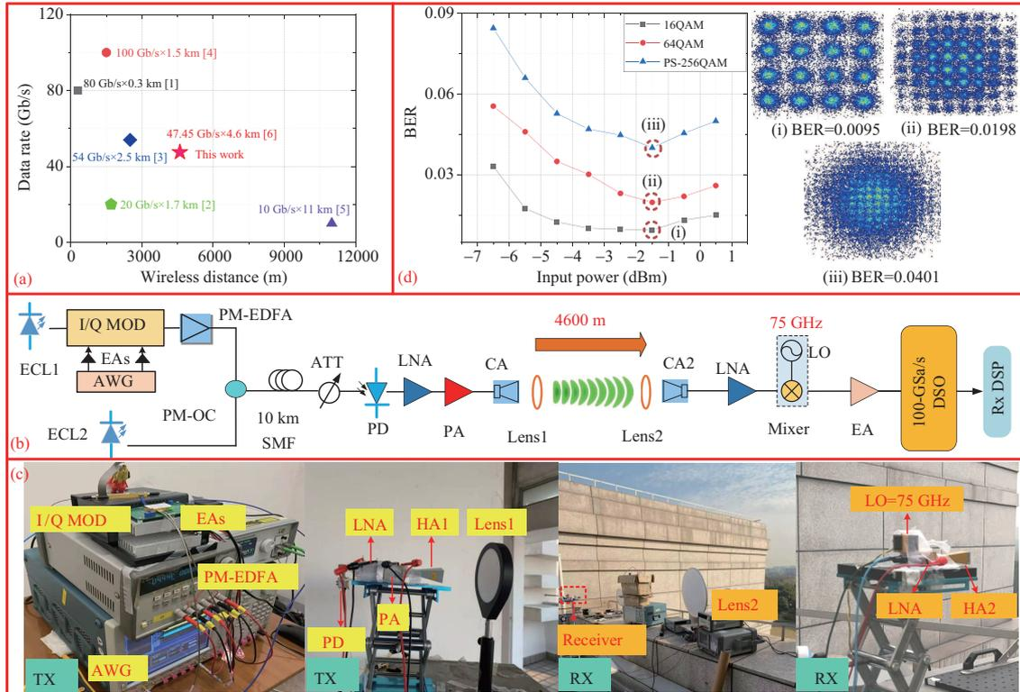
**Figure 1** (Color online) (a) The important experimental demonstrations of high-speed long-distance transmission at the W-band; (b) experimental setup; (c) the photos of the transceiver; (d) BER curve of 9.6 Gbaud QAM signal.
