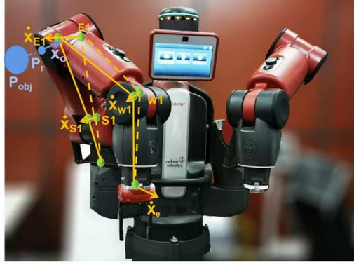
**Figure A1** The motion of each joint angle during obstacle avoidance.
