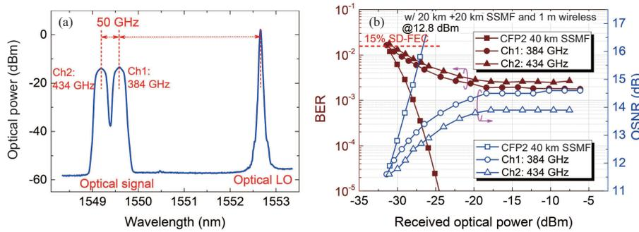
**Figure 10** (Color online) Test results of the 200 GbE real-time fiber-THz-fiber transmission. (a) Spectra at the O-T side; (b) BER and OSNR versus received optical power for two channels.
