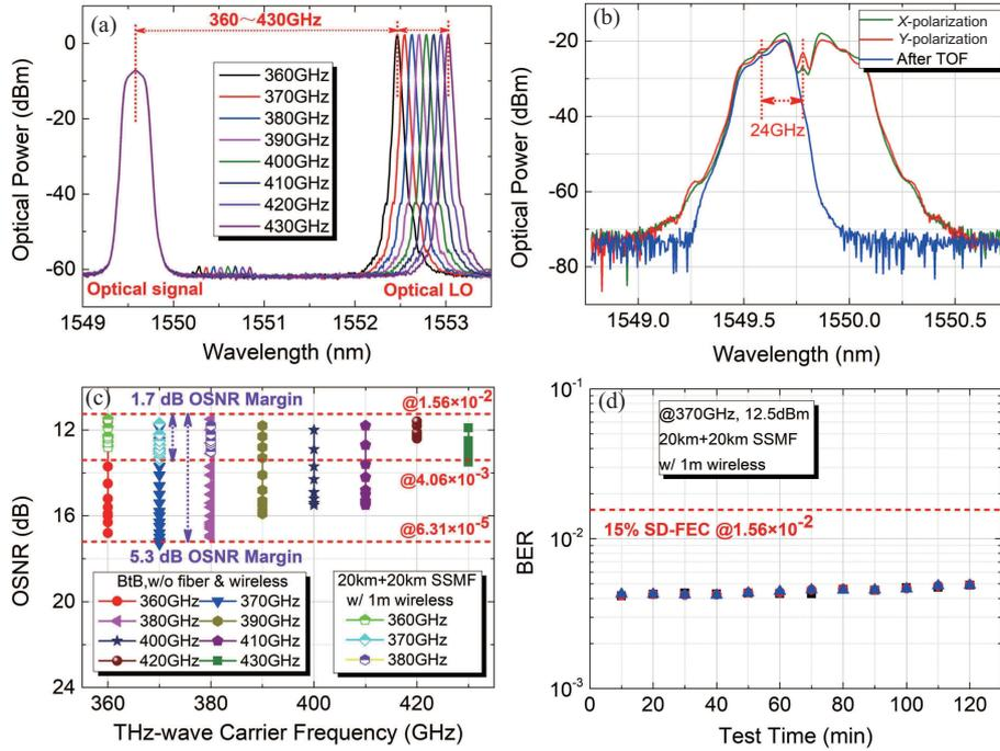
**Figure 9** (Color online) Test results of the 100 GbE real-time fiber-THz-fiber transmission. (a) Spectra at the O-T side; (b) spectra at the T-O side; (c) performance of OSNR; (d) transmission stability test results [51, 52].
