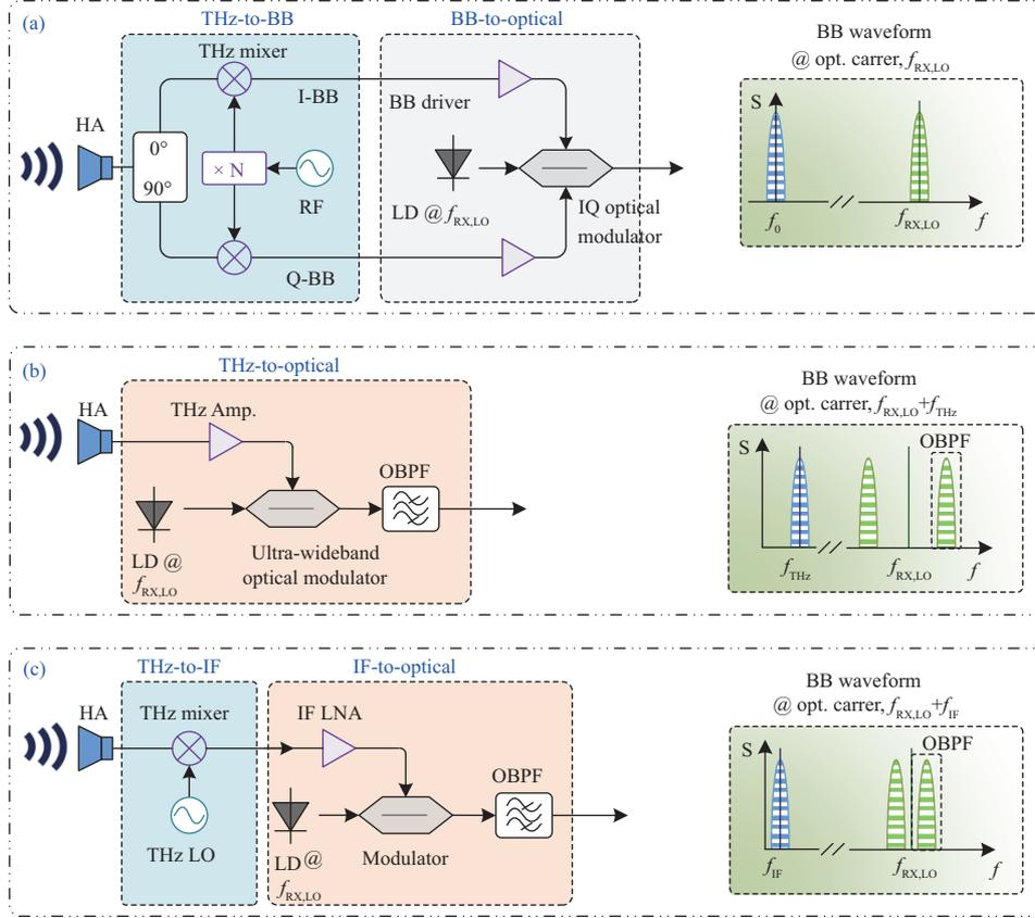
**Figure 3** (Color online) THz down-conversion techniques. (a) All-electric down-conversion; (b) all-optical down-conversion; (c) hybrid optoelectronic down-conversion.
