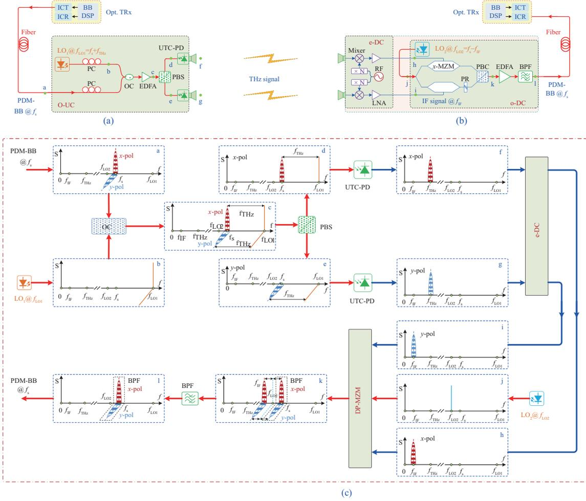
**Figure 5** (Color online) Key modules. (a) O-T conversion module; (b) T-O conversion module; (c) spectra diagram of up-conversion and down-conversion.
