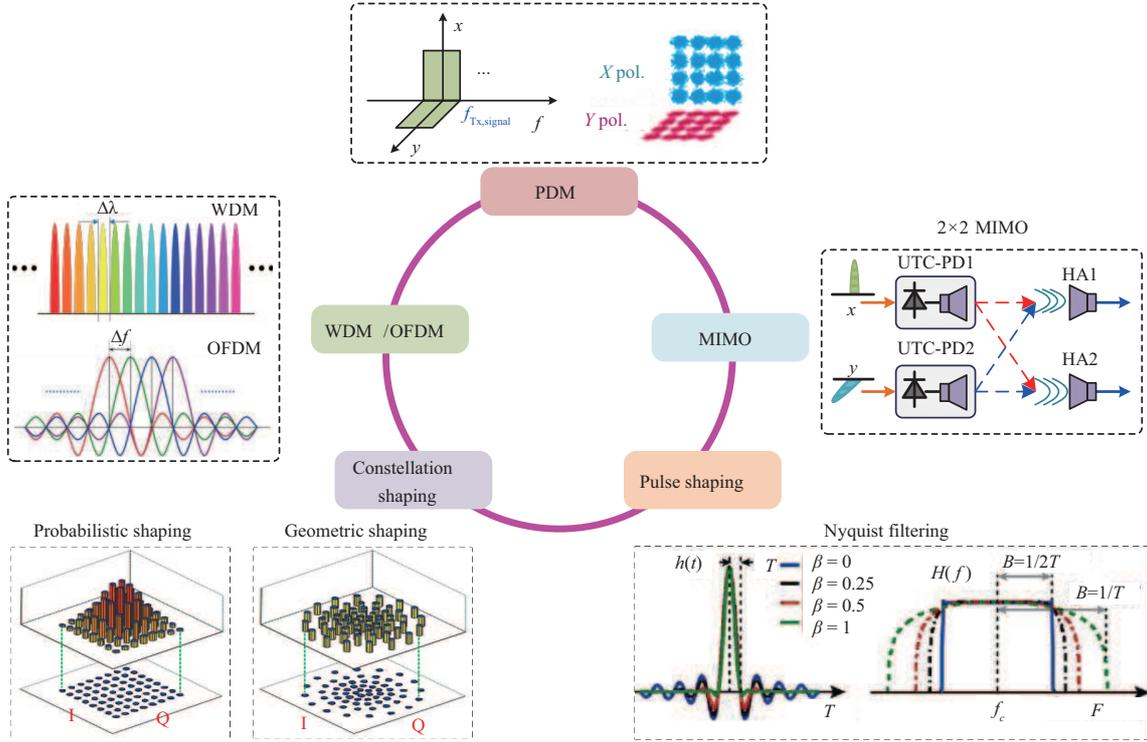
**Figure 6** (Color online) Five dimensions of high spectral efficiency and ultra-wideband THz signal modulation.
