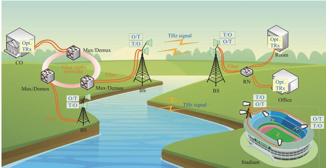
**Figure 4** (Color online) Fiber-THz-fiber seamlessly converged system architecture.
