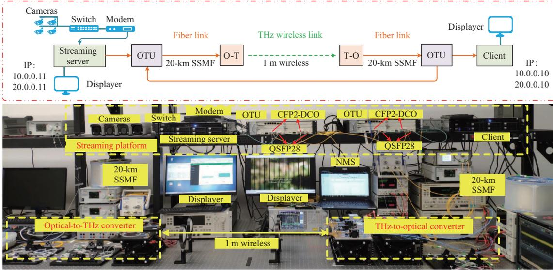
**Figure 8** (Color online) Demonstration of the 100/200 GbE real-time transparent fiber-THz-fiber  $2 \times 2$  MIMO transmission system [50].
