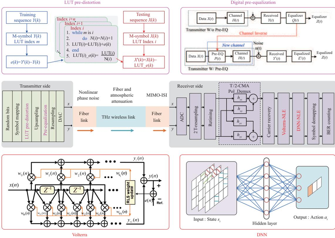
**Figure 7** (Color online) Intelligent nonlinear damage compensation techniques for THz-fiber hybrid channels.
