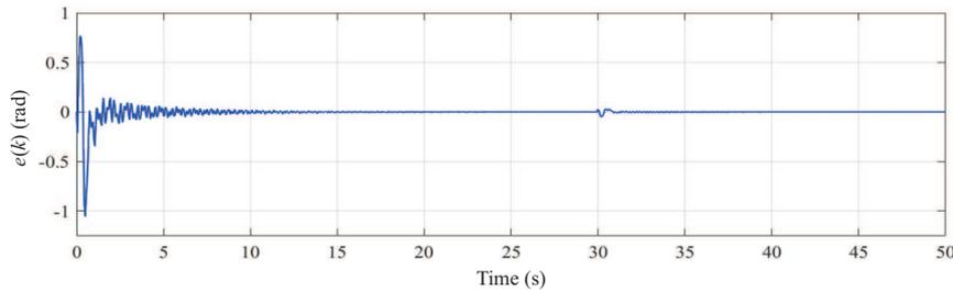
**Figure 13** (Color online) Tracking error  $e(k)$  of the controlled-system with 10% plant variation.
