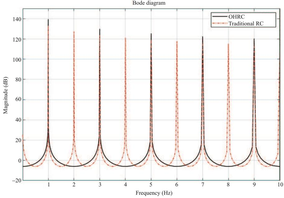
**Figure 1** (Color online) Magnitude responses of the internal models of OHRC and traditional RC with a fundamental frequency of 1 Hz.
