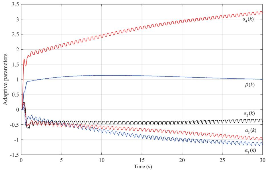
**Figure 9** (Color online) Adaptive parameters  $\alpha(k)$  and  $\beta(k)$  of RAC.
