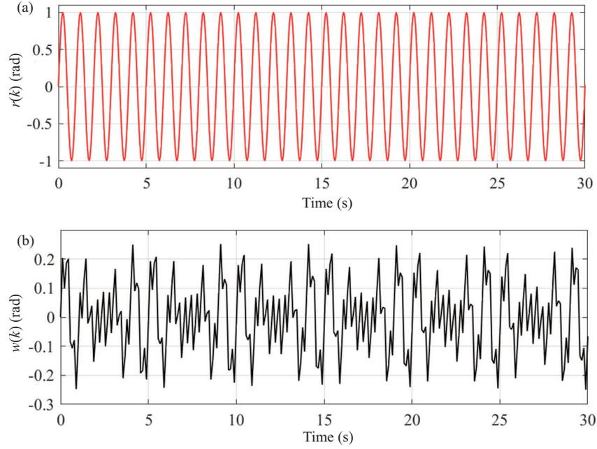
**Figure 3** (Color online) (a) Reference  $r(k)$ ; (b) disturbance  $w(k)$ .
