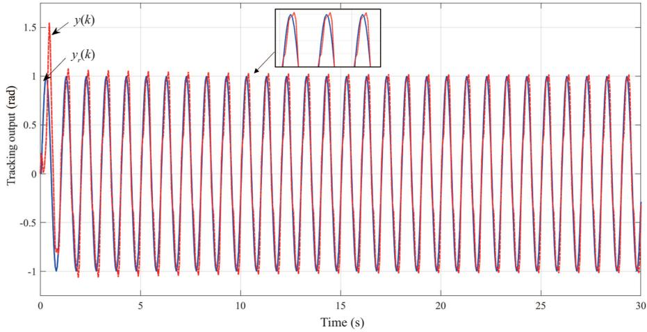
**Figure 11** (Color online) Plant output  $y(k)$  and reference output  $y_r(k)$  of RAC.
