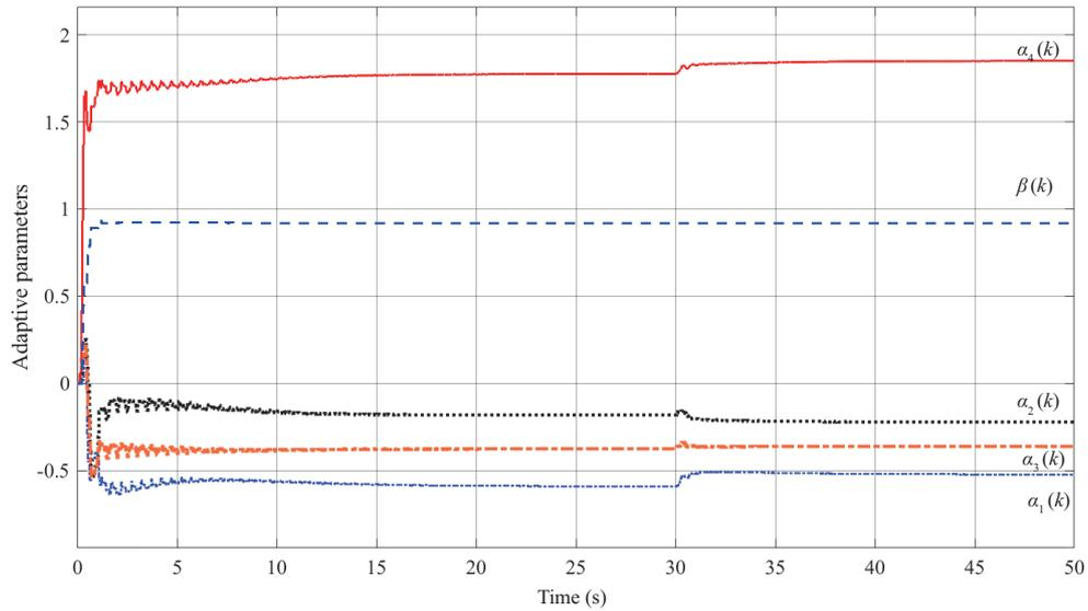
**Figure 12** (Color online) Adaptive parameters  $\alpha(k)$  and  $\beta(k)$  of the controlled-system with 10% plant variation.
