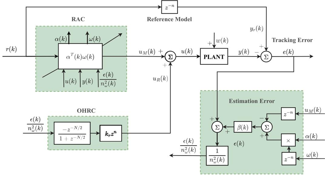
**Figure 2** (Color online) A closed-loop system with the proposed RA-OHRC.
