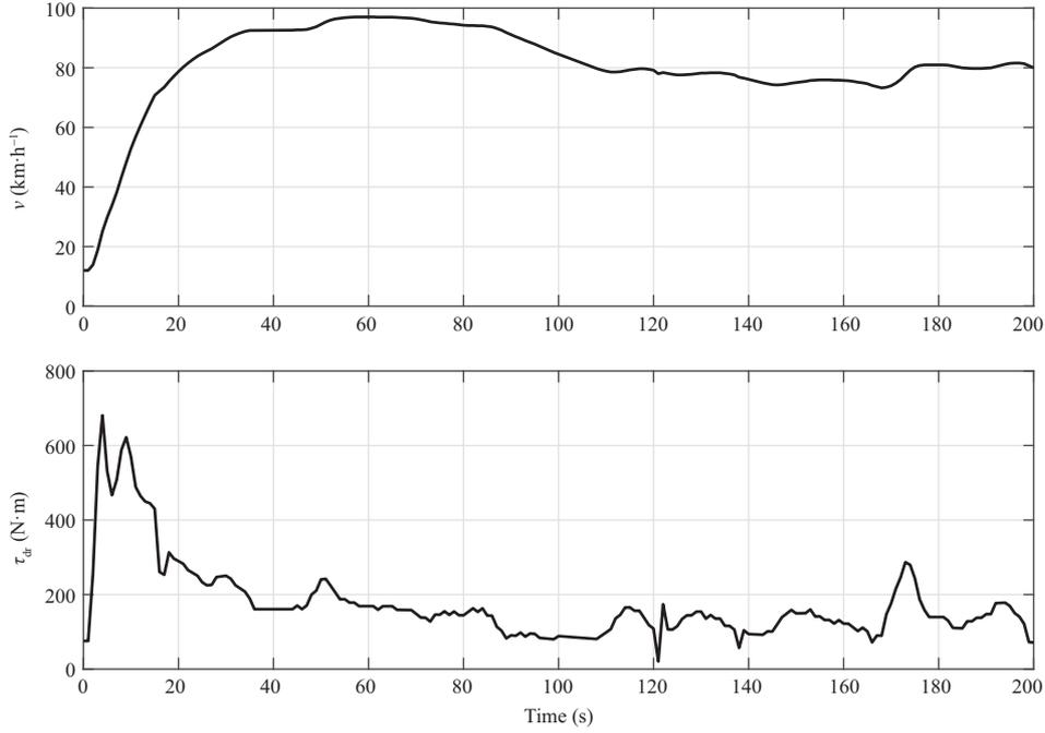
Figure 4 Testing scenario data: vehicle speed trajectory and driving torque demand.
