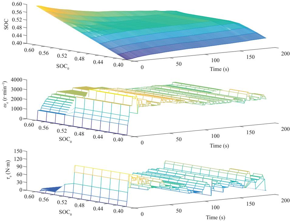
**Figure 7** (Color online) State trajectories and solutions under different initial state values:  $D_{SOC} = 0.31 \times 10^{-2}$ ,  $D_{\tau_e} = 8.8$ ,  $D_{\omega_e} = 219$ .
