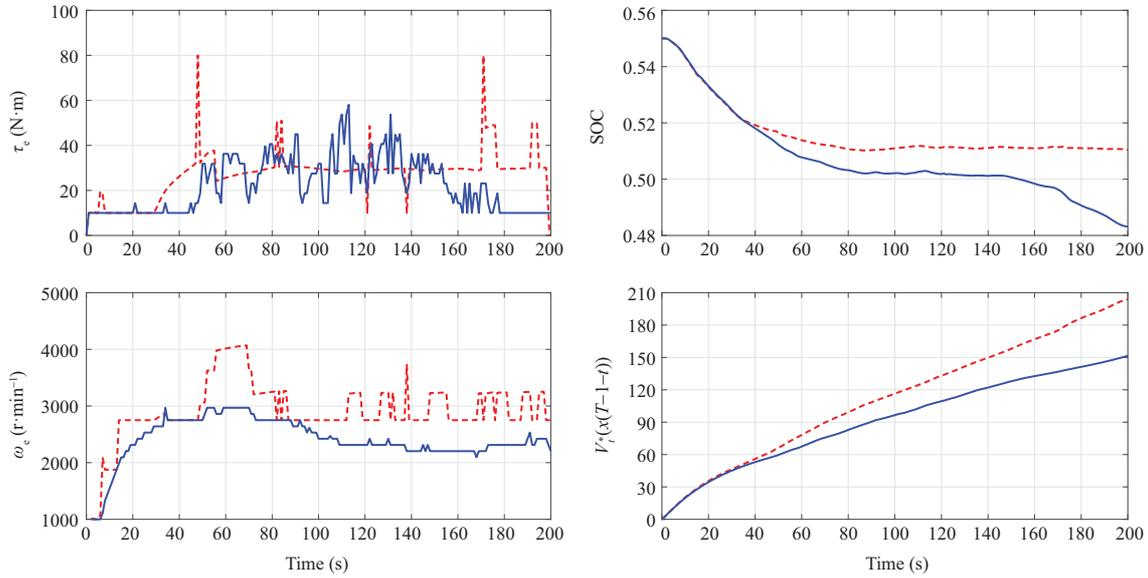
**Figure 6** (Color online) Results of 2 cases by the logical control strategy (dashed line:  $D_{\text{SOC}} = 2.5 \times 10^{-2}$ ,  $D_{\omega_e} = 875 \text{ r} \cdot \text{min}^{-1}$ ,  $D_{\tau_e} = 35 \text{ N} \cdot \text{m}$ ; solid line:  $D_{\text{SOC}} = 0.02 \times 10^{-2}$ ,  $D_{\omega_e} = 109 \text{ r} \cdot \text{min}^{-1}$ ,  $D_{\tau_e} = 4.4 \text{ N} \cdot \text{m}$ )
