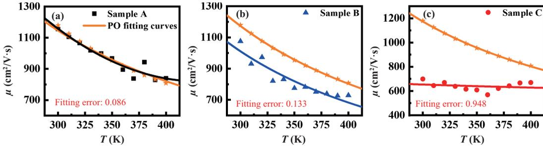
**Figure 7** (Color online) Statistical peak field-effect mobility of (a) sample A, (b) sample B, and (c) sample C as a function of temperature (geometries) and fit curves by using the optical phonon scattering model (lines).
