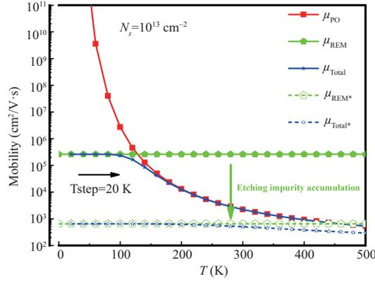
**Figure 6** (Color online) Relationship of the scattering mobility and temperature when the 2DEG density is  $1.0 \times 10^{13} \text{ cm}^{-2}$ .
