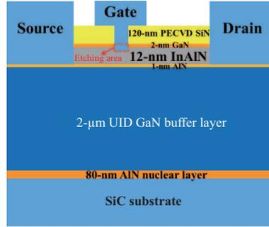
**Figure 1** (Color online) Schematic cross-section of a recessed-gate InAlN/GaN HEMT.
