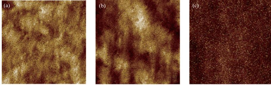
**Figure 2** (Color online) AFM surface morphology (area:  $8 \times 8 \mu\text{m}^2$ ) of InAlN/GaN samples (a) without ICP etching, (b) with ICP etching, and PET (c) with ICP etching.
