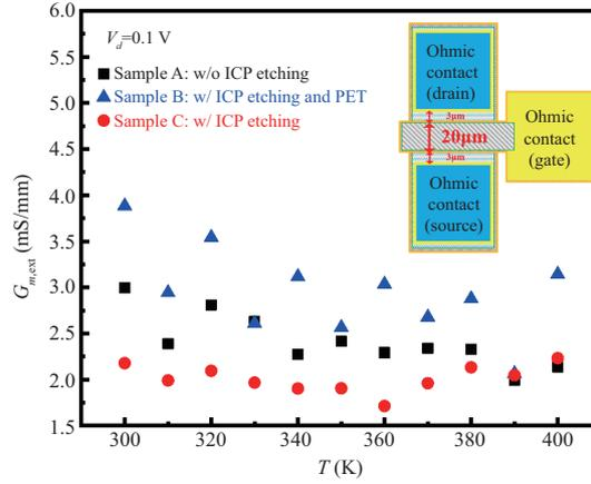
**Figure 5** (Color online) Top view of the devices and perform variable temperature ( $T$ ) test on samples A, B, and C.
