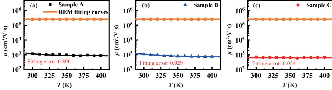
**Figure 8** (Color online) Statistical peak field-effect mobility of sample A (a), sample B (b), and sample C (c) as a function of temperature (geometries) and fit curves by using the remote charge scattering model (lines).
