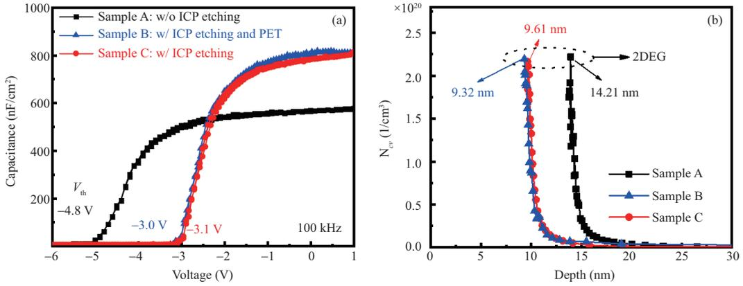
**Figure 4** (Color online) (a)  $C$ - $V$  characteristics at a frequency of 100 kHz: for sample A device without recessed gate and for samples B and C with recessed gate. (b) 2DEG distribution ( $N_{CV}$ ) versus depth for samples A, B, and C.
