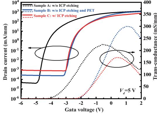
**Figure 3** (Color online) Transfer curves of the planar-gate device (sample A), recessed-gate device by ICP etching with PET (sample B), and ICP etching (sample C).
