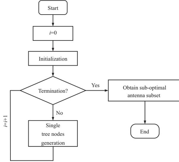
Figure 4 Flowchart depicting the structure of STSAS used in the OSM system.
