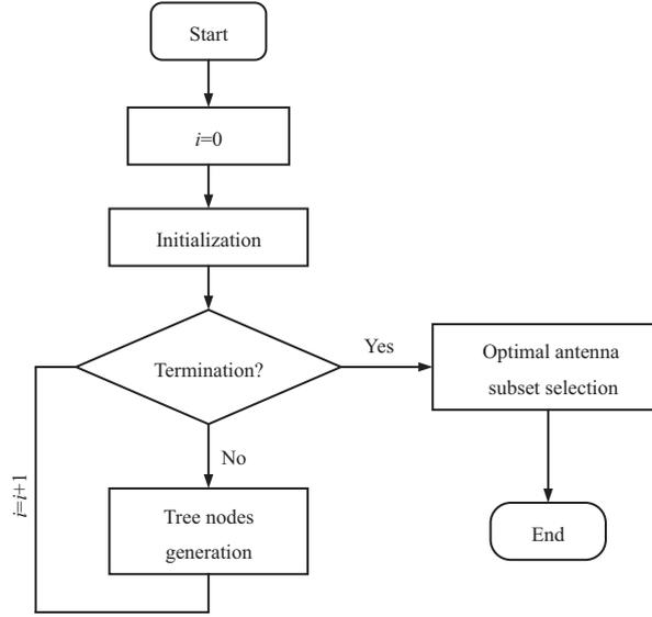
**Figure 2** Flowchart depicting the structure of TSAS used in the OSM system.
