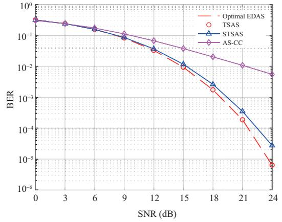
**Figure 7** (Color online) BER performance of the optimal EDAS, TSAS, STSAS, AS-CC schemes in a QPSK scenario employing  $N_r = 1$ ,  $N_s = 8$  and  $N_t = 17$ .
