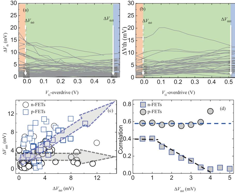
**Figure 1** (Color online) The experimental relationship between  $V_G$ -overdrive ( $V_G - V_{th0}$ ) and threshold voltages fluctuation in (a) n-FETs and (b) p-FETs, respectively. (c) The relationship between  $\Delta V_{th0}$  and  $\Delta V_{thH}$  and (d) the autocorrelation coefficient under various  $\Delta V_{th0}$  for n-FETs and p-FETs, respectively.
