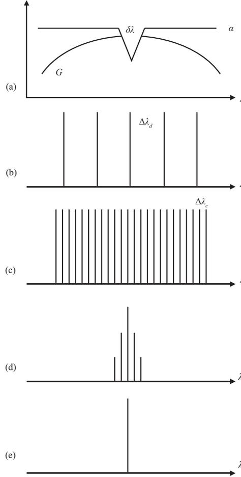
**Figure 4** Schematic of Littman-ECDL mode selection. (a) Gain-medium gain curve and loss curve; (b) gain chip spectrogram; (c) external-cavity spectrogram; (d) gain-saturation competition; (e) mode competition results in a single longitudinal mode.
