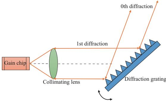
**Figure 2** (Color online) Schematic of Littrow-ECDL.
