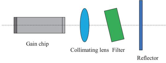
**Figure 5** (Color online) Schematic of filter-ECDL.
