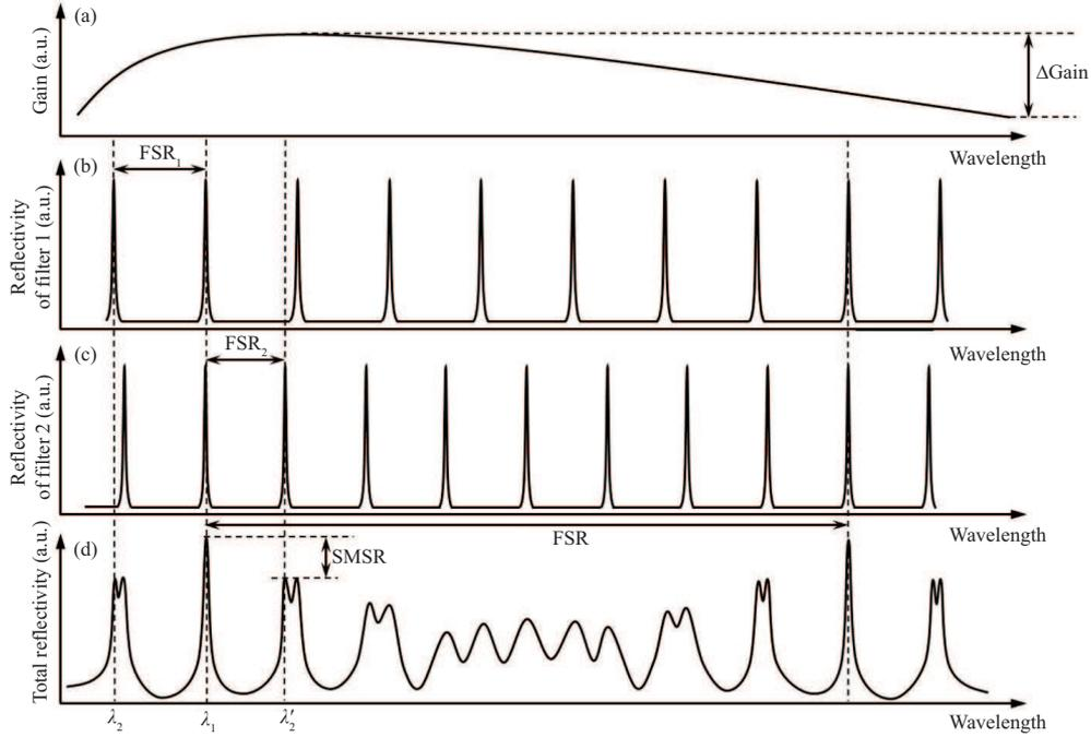
**Figure 7** Schematic of MRR-ECDL mode selection based on cursor effect. (a) Gain-medium gain curve; (b) “filter 1” comb spectrum; (c) “filter 2” comb spectrum; (d) superimposed spectra of two filters.
