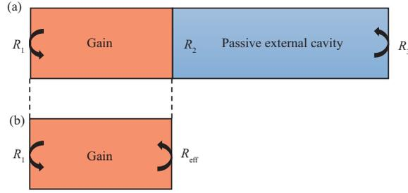
**Figure 1** (Color online) (a) ECDL model and (b) equivalent cavity surface model.
