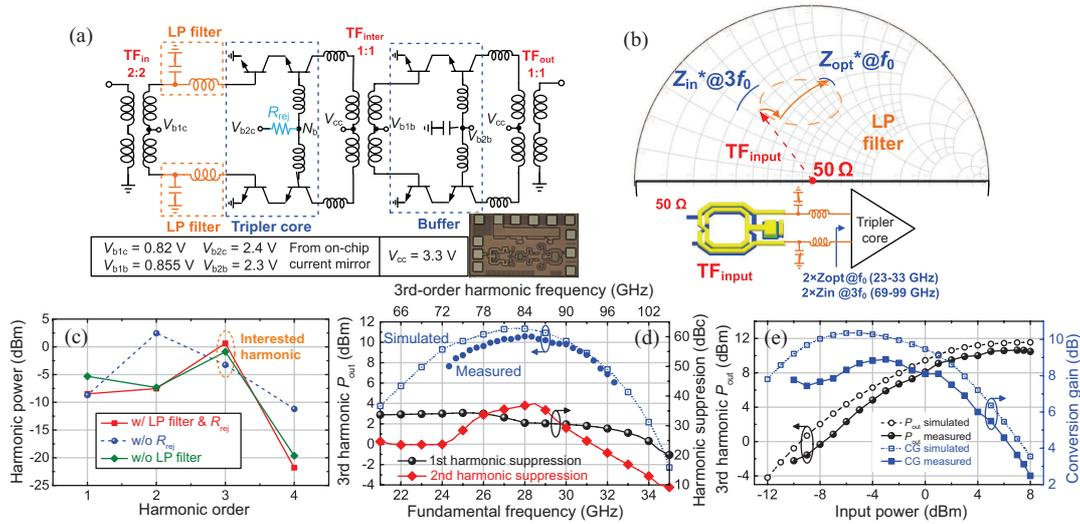
**Figure 1** (Color online) (a) Schematic of the frequency tripler; (b) impedance transformation of the input matching network (the trajectory of the transformer is simplified); (c) simulated harmonic power at the output of the tripler core; (d) output power and harmonic suppression with the input power of 5 dBm; (e) output power and conversion gain with the fundamental frequency of 28 GHz.
