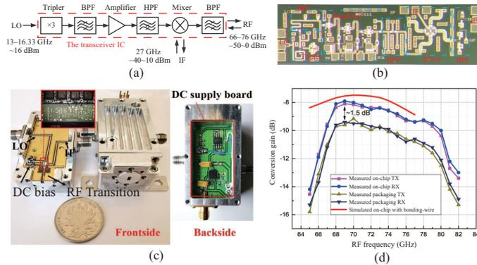
**Figure 1** (Color online) (a) Block diagram of the transceiver MMIC (with frequency and power budget); (b) photograph of the MMIC (chip size: 2.7 mm × 0.9 mm); (c) photograph of the opened split-block and assembled module including MMIC and RF microstrip-to-waveguide transition; (d) simulated and measured conversion gain of the chip and module.
