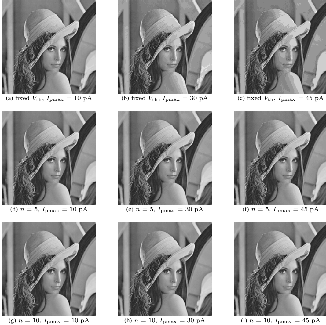
Figure C4 The reconstructed images. (a), (b), and (c) are images reconstructed based on fixed threshold, with maximum mapping current 10 pA, 30 pA, and 45 pA, respectively. (d), (e), and (f) are images reconstructed based on variable threshold and window depth 5, with maximum mapping current 10 pA, 30 pA, and 45 pA, respectively. (g), (h), and (i) are images reconstructed based on variable threshold and window depth 10, with maximum mapping current 10 pA, 30 pA, and 45 pA, respectively.
