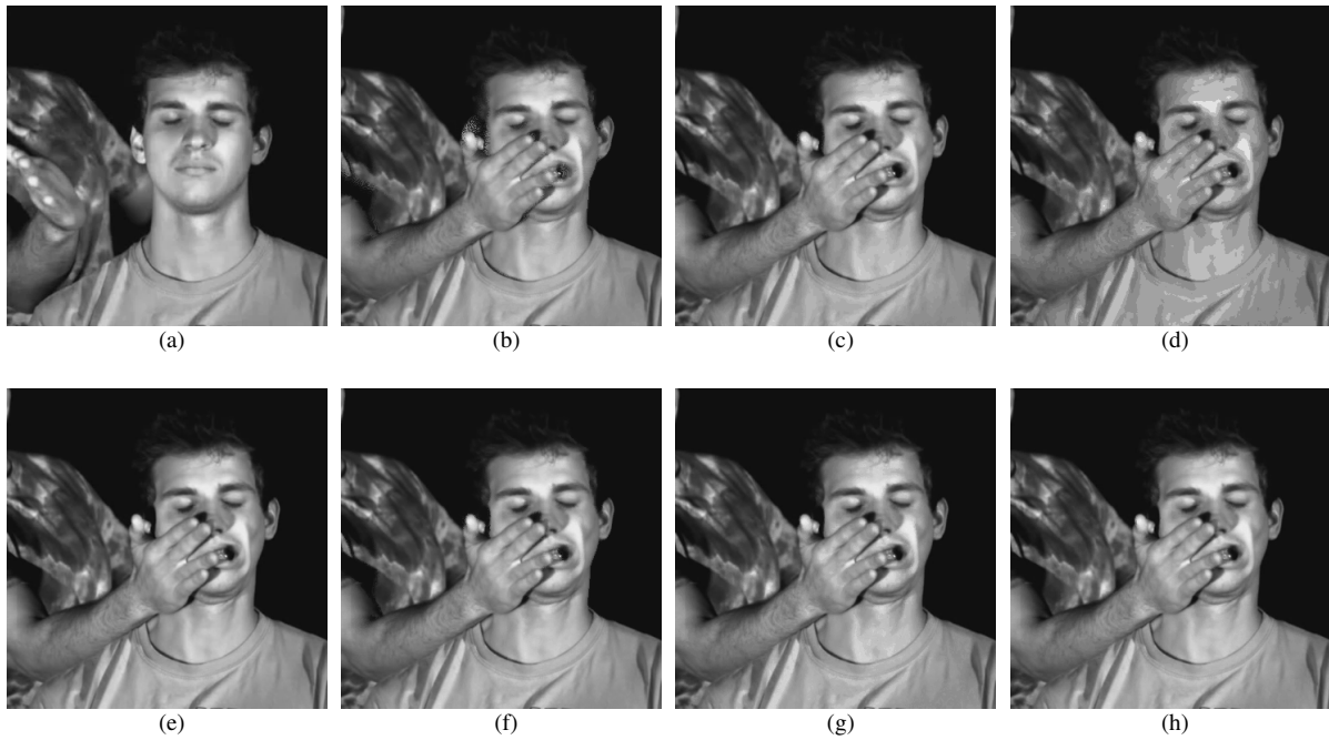
Figure C7 A frame of the video. (a) is the first frame of the original video. (b), (c), and (d) are the reconstructed frame based on fixed threshold with I_{pmax} set to 3 pA, 15 pA and 45 pA, respectively. (e) is the frame of the original video corresponding to the reconstructed frame shown in other sub images. (f), (g), and (h) are the reconstructed video based on variable threshold with I_{pmax} set to 3 pA, 15 pA and 45 pA, respectively.
