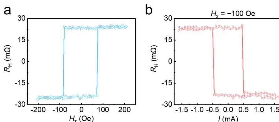
**Figure S1.** Deterministic switching of the nanomagnets induced by (a) OOP fields and (b) SOT with the assistance of an IP field.
