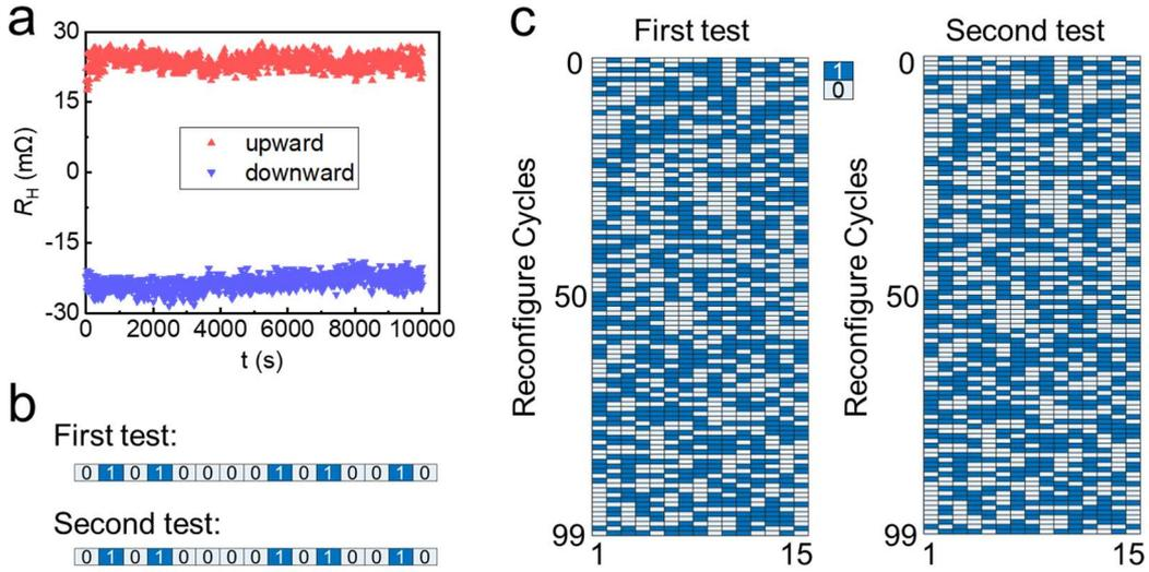
**Figure S4** (a) Retention characteristic of the two different resistance levels, measured under 50  $\mu$ A read current for  $10^4$  s. (b) Bitmaps of 1  $\times$  15 binary bits for two tests. (c) Bitmaps of 100  $\times$  15 binary bits for two tests.
