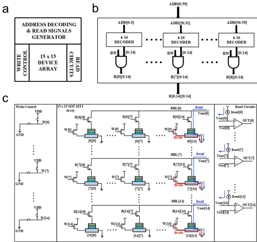
**Figure S9.** Circuit scheme of the CMOS/SOT-MTJ based RPUF: (a) block diagram, (b) block of
