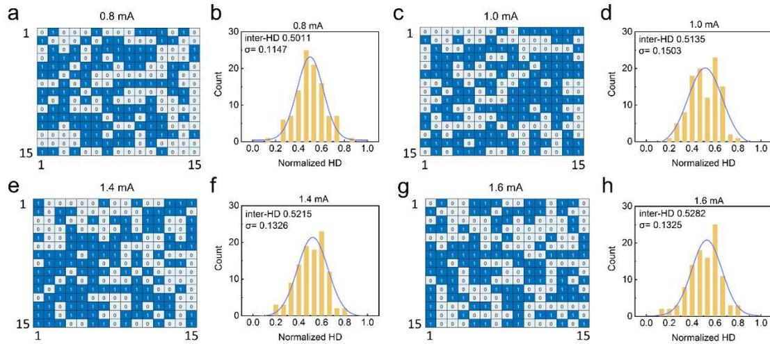
**Figure S5.** Bitmaps and inter-HDs of RPUFs under different writing currents.
