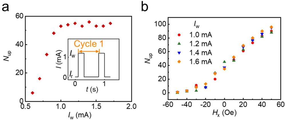
**Figure S2.** Switching probability under different (a) current amplitudes  $I_w$  and (b) IP fields  $H_x$ .
