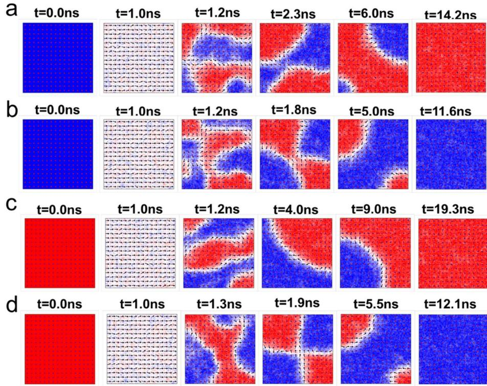
**Figure S3.** Object-Oriented Micro-Magnetic Framework micromagnetic simulations of the magnetization evolution based on the generalized Landau–Lifschitz–Gilbert theory, using a current density of  $5 \times 10^{12} \text{ A/m}^2$  (1 ns). Red (blue) for positive (negative) OOP component, while the arrows indicate the IP component of the magnetization.
