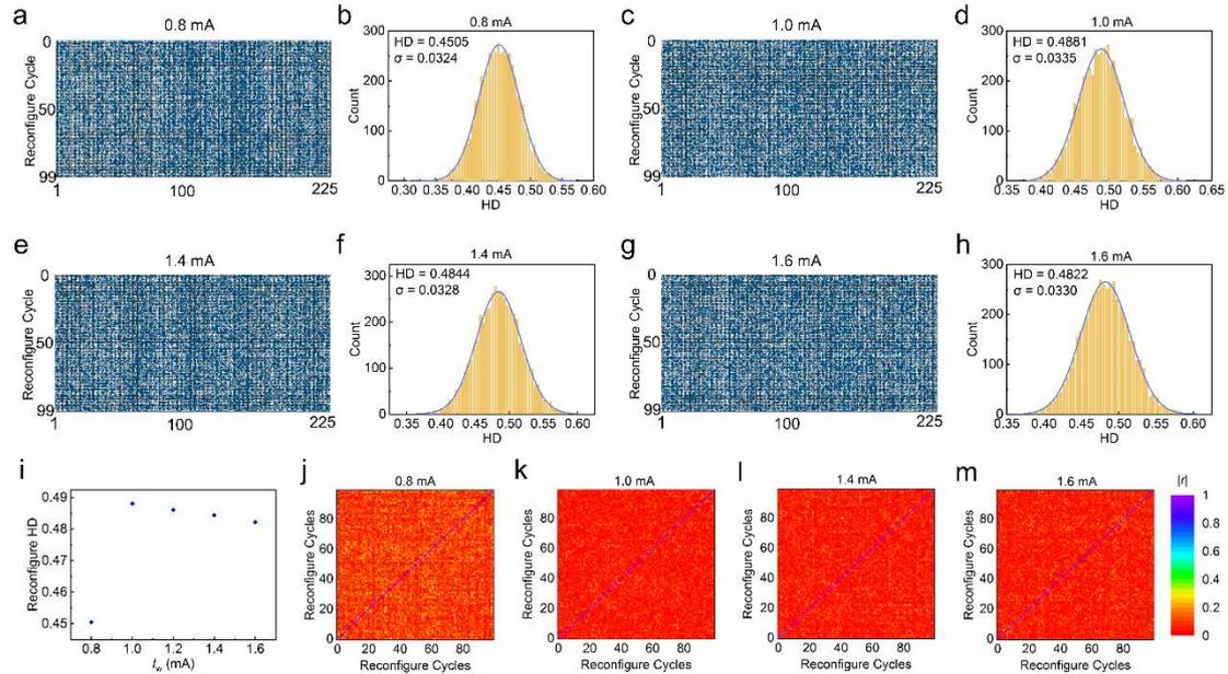
**Figure S7.** Evaluation of reconfigurability of the RPUF under a series of writing currents. (a)(c)(e)(g) Bitmaps of  $225 \times 100$  binary bits after 100 reconfigure cycles. (b)(d)(f)(h) Reconfigure-HDs distribution between 100 reconfigured keys with Gauss fitting (blue line). (i) Mean Reconfigure-HDs as a function of currents. (j-m) Correlation matrix of 100 reconfigured keys.
