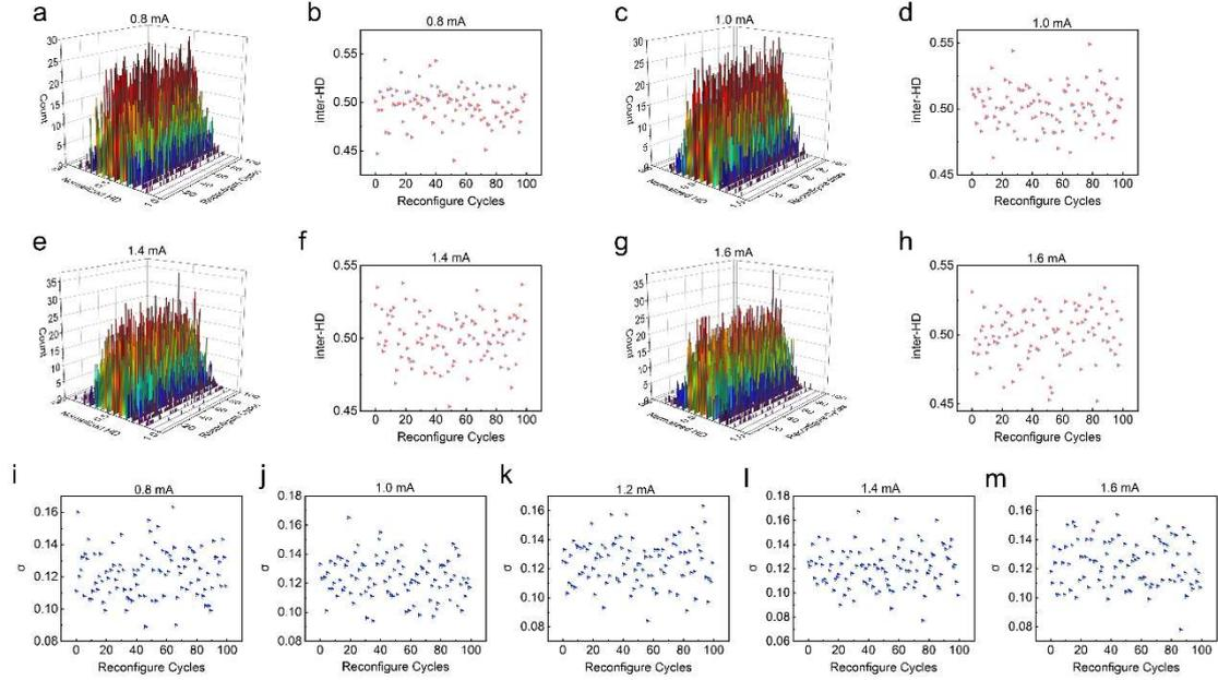
**Figure S6.** Distribution of the HDs of 100 reconfigure cycles under different writing currents. (a-h) Inter-HDs of 100 reconfigure cycles with their mean values and (i-m) standard deviations extracted from Gaussian function fitting under different writing currents.
