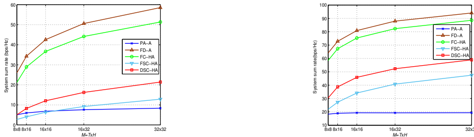
Figure E5 System sum rate versus M for different architecture with SNR=-5 (dB) Figure E6 System sum rate versus M for different architecture with SNR=10 (dB)
