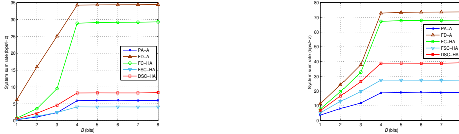
Figure E3 System sum rate versus B for different architectures with SNR=-5 (dB) Figure E4 System sum rate versus B for different architectures with SNR=10 (dB)
