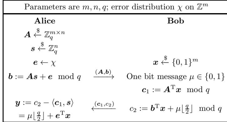
**Figure 1** An example of LWE-based public-key encryption.
