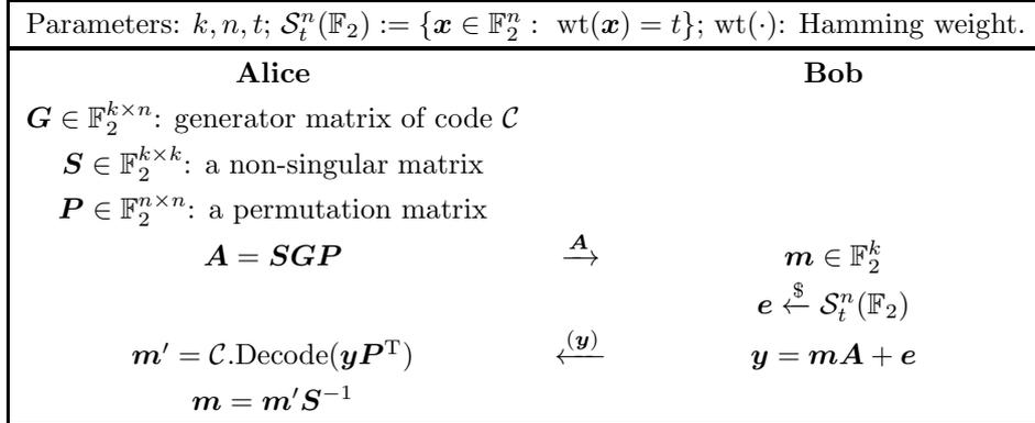
Figure 5 Illustration of McEliece public-key encryption scheme.
