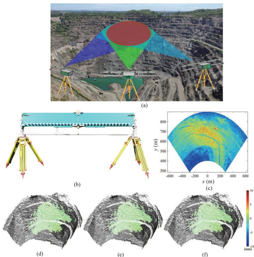
**Figure 1** (Color online) (a) Measurement geometry of a 3D deformation; (b) GB-MIMO radar; (c) radar image; (d) deformation along the  $x$ -axis; (e) deformation along the  $y$ -axis; (f) deformation along the  $z$ -axis.
