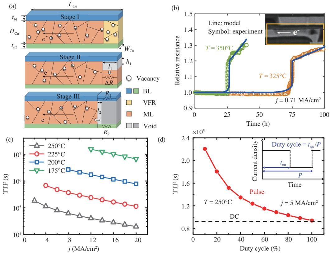
**Figure 1** (Color online) (a) Physics-based EM reliability model of interconnects, which accounts for the process of resistance evolution; (b) modeling resistance evolution in comparison of experimental data [7]; (c) EM lifetime prediction with different operation current densities; (d) EM lifetime in pulse operation with different duty cycles.
