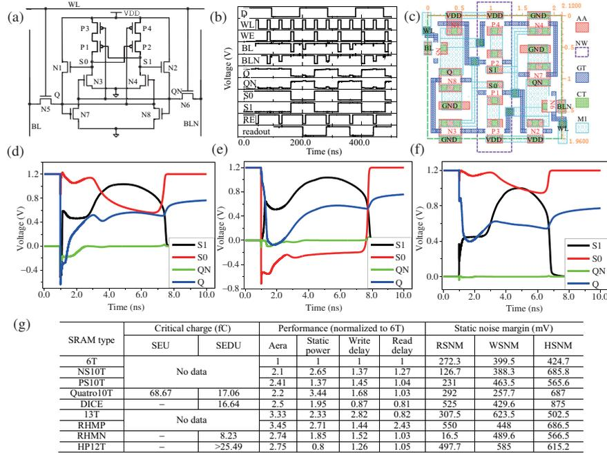
**Figure 1** (Color online) (a) Schematic diagram of the proposed HP12T SRAM cell; (b) normal operation diagram of HP12T SRAM cell; (c) the layout of HP12T SRAM cell; (d) ion striking on node Q; (e) ion striking on node S0; (f) ion striking on node S1; (g) comparisons of different SRAMs' performance (please refer to [1] for understanding the structure of each SRAM cell listed here).
