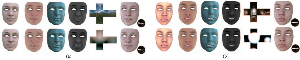
Figure 11 (Color online) Comparisons with the ground truth. The 1st row is the ground truth, the 2nd row is our result. For each row from left to right in (a) and (b): the target images or the rendering of our reconstruction, albedo, normal, specular, environmental lighting, and a relighting result.
