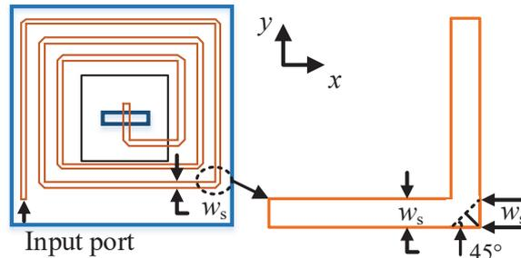
**Fig. A2** Details of the shear corner in the power divider network.
