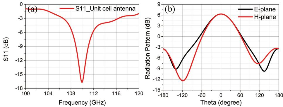
**Fig. A1** Simulated results of the designed antenna unit based on NLCs. (a) The result of S-parameter from 100 to 120GHz. (b) The 2D radiation beams of the designed antenna unit at 110GHz.
