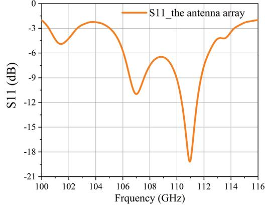
**Fig. B1** S-parameter simulation results array antenna based on NLCs from 100 to 116GHz.
