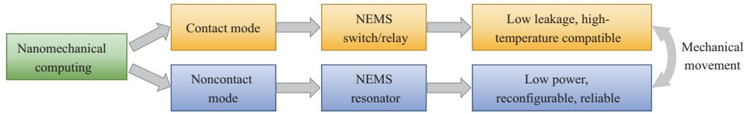
**Figure 1** (Color online) Two categories of nanomechanical computing devices and their respective advantages.
