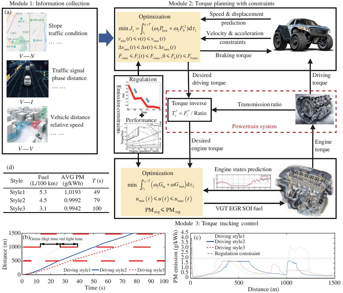
**Figure 1** (Color online) Simulation results under three different driving styles. (a) Overall structural schematic flow chart; (b) driving route; (c) PM emissions; (d) analysis of experimental data.
