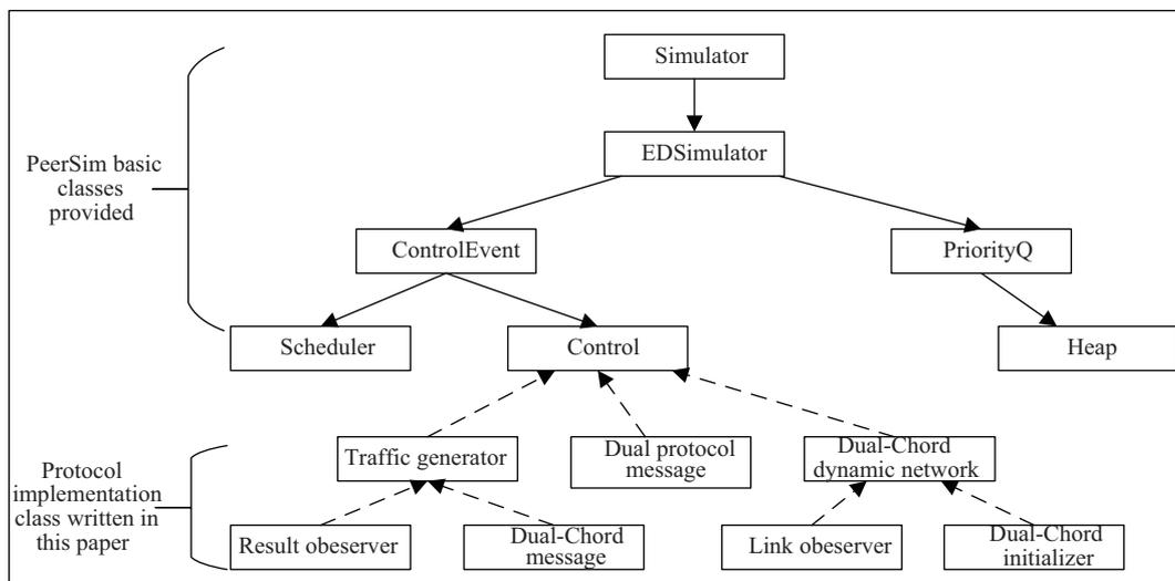
Figure 5 File structure of simulation code.
