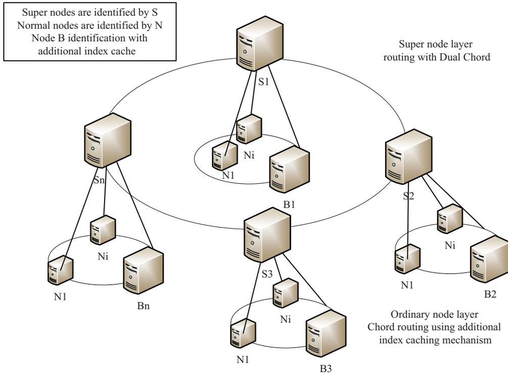
**Figure 3** (Color online) Model diagram of two-level identification analysis system based on improved Chord algorithm.
