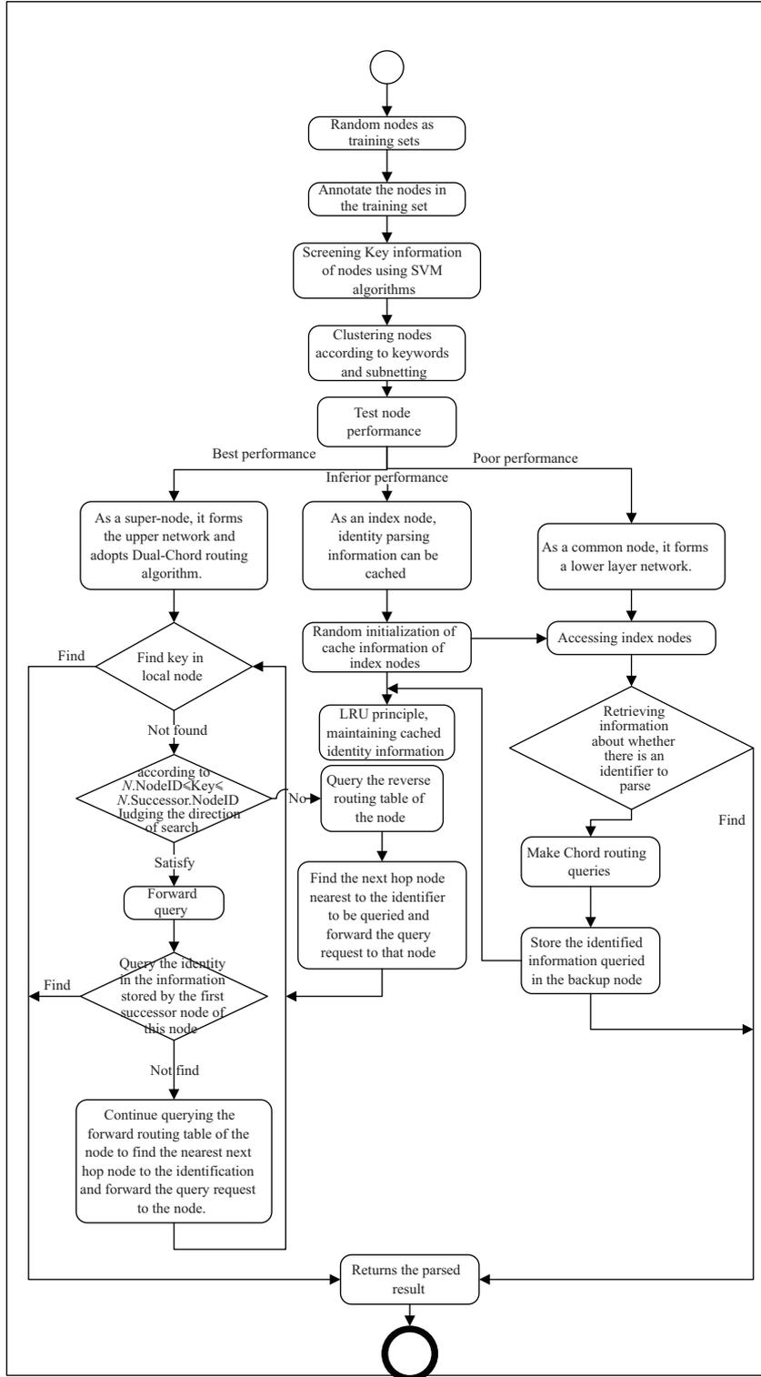
Figure 4 Workflow diagram of two-level identity resolution system.
