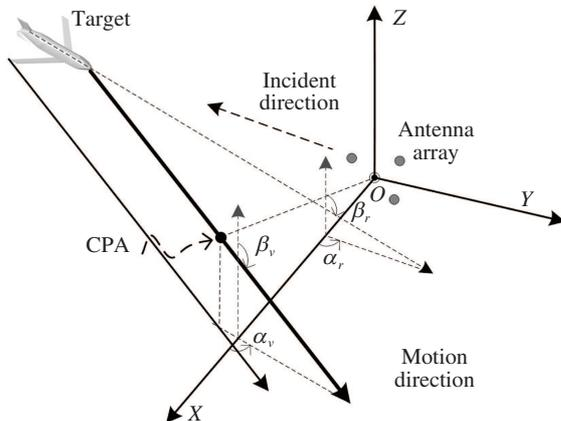
**Figure 1** Geometrical relation of the approaching object and a measuring antenna array.
