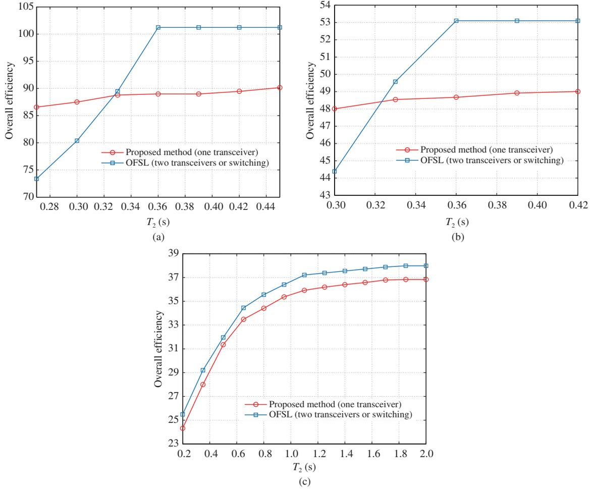
**Figure 9** (Color online) The comparison between the proposed method and OFSL with  $T_1 = 0.2$  s under three trajectories. (a) Carpet; (b) Troop; (c) Ring.
