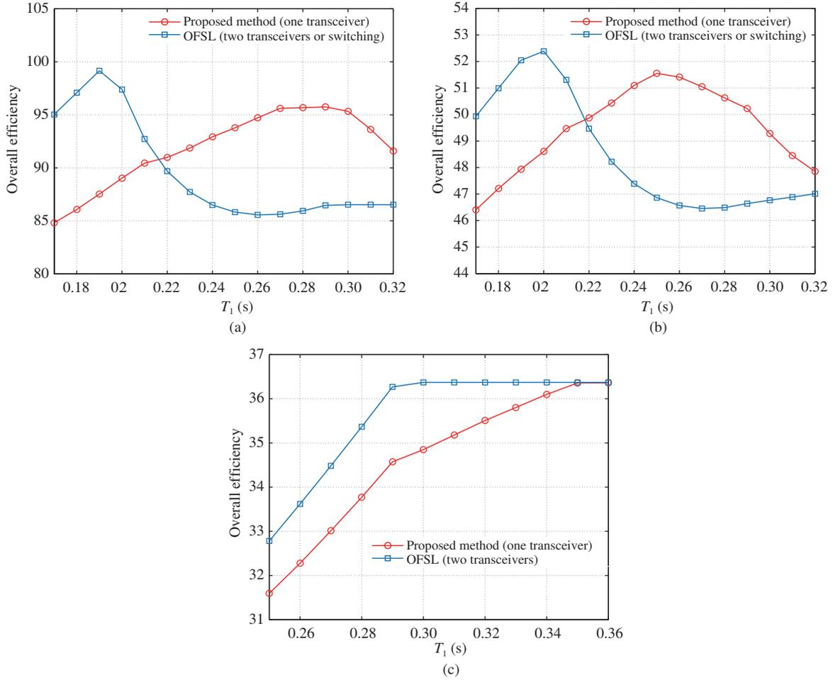
**Figure 8** (Color online) The comparison between the proposed method and OFSL with  $T_2 = 0.35$  s under three trajectories. (a) Carpet; (b) Troop; (c) Ring.
