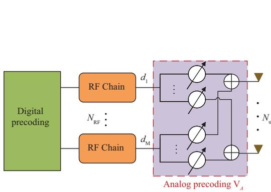
**Figure 2** (Color online) Fully-connected hybrid precoding for mmWave NOMA-UAV networks.
