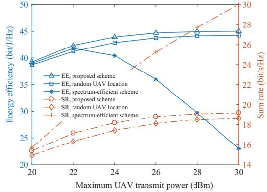
**Figure 7** (Color online) Energy efficiency and sum rate comparison between the proposed scheme and two benchmarks.
