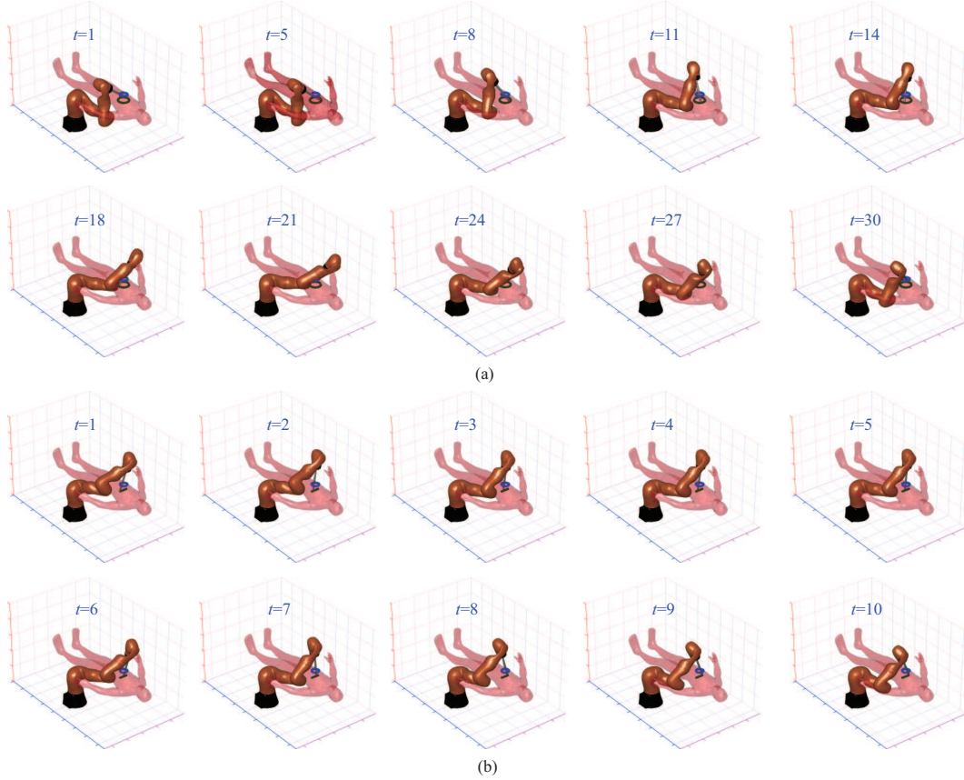
Figure 10 (Color online) Simulation results for (a) circular reference trajectory with \Lambda = 2.5 and (b) linear reference trajectory with \Lambda = 3 .
