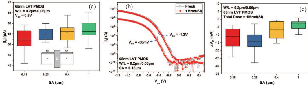
**Figure 1** (Color online) (a) Box-plot of the drain current of PMOS devices as a function of SA values at the same overdrive voltage ( $V_{ov} = 0.6\text{V}$ ). The inset shows the definition of SA. (b) The typical transfer characteristic curves of 65-nm PMOS device with SA of 0.18  $\mu\text{m}$  before and after irradiation. (c) Box-plot of  $V_{th}$  shift as a function of SA values after 1 Mrad(Si) TID irradiation.
