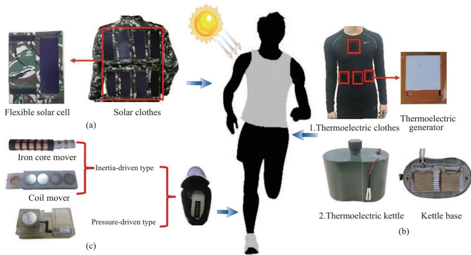
**Figure 1** (Color online) Ubiquitous energy harvesting devices. (a) Solar energy harvesting device; (b) thermal energy harvesting device; (c) foot mechanical energy harvesting device.
