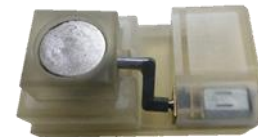
Foot mechanical energy harvesting device
