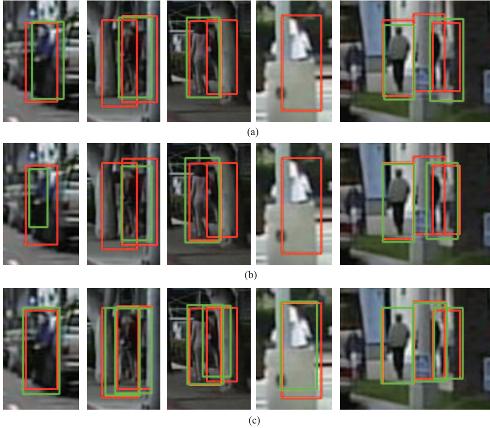
Figure 6 (Color online) Qualitative detection comparison of (c) PSC-Net with (a) AR-Ped [7] and (b) MGAN [13] under occlusions on Caltech test images. Here, all detection results are obtained using the same false positive per image criterion. The red boxes denote the ground-truth whereas the detector's predictions are marked in green.
