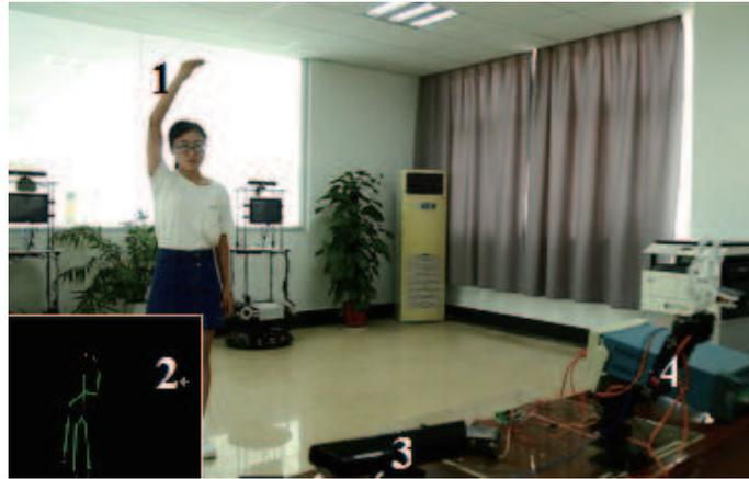
**Figure 4** (Color online) Experimental environment. 1: the human arm, 2: the data-processing PC used to obtain the gesture data, 3: Kinect, 4: robotic arm.
