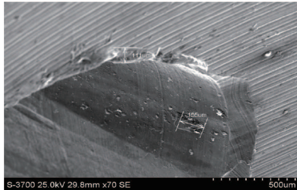
Figure 6 Illustration of a deformed motor bearing.
