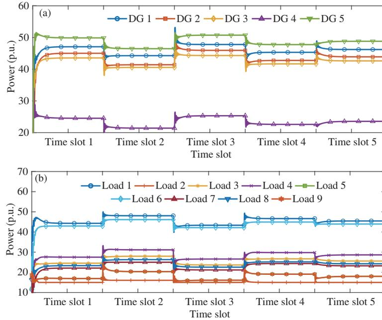
**Figure 3** (Color online) (a) Power output of the distributed generators; (b) load demand of the users.
