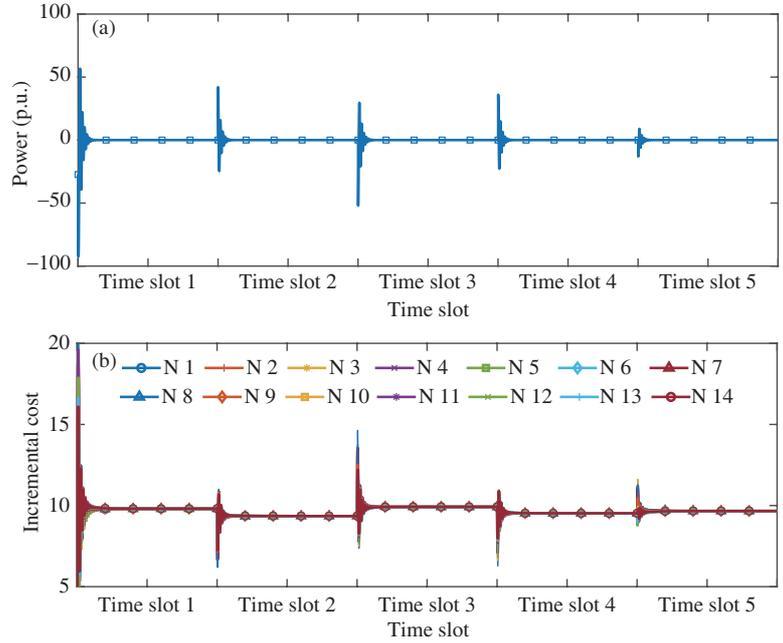
Figure 4 (Color online) (a) Mismatch of entire grid and (b) the incremental cost of each generation in five time slots.
