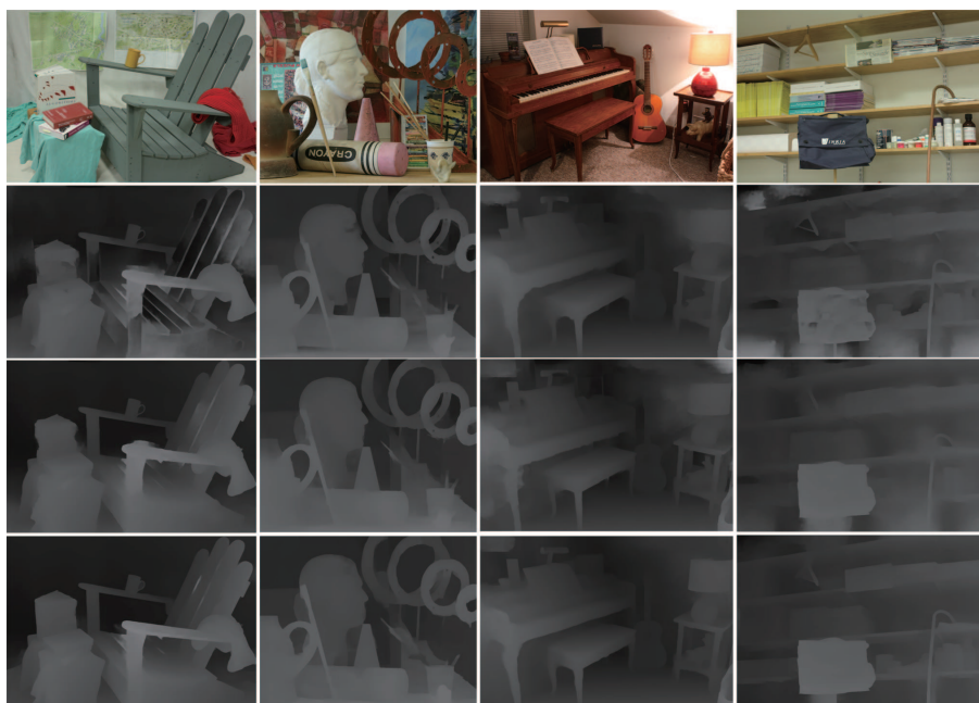
Figure 4 (Color online) Disparity maps achieved by StereoNet. The 1st row shows the color images in the training set of Middlebury 2014, the 2nd row shows the results of StereoNet-A, the 3rd row shows the results of StereoNet-C, and the last row shows the results of StereoNet-E.
