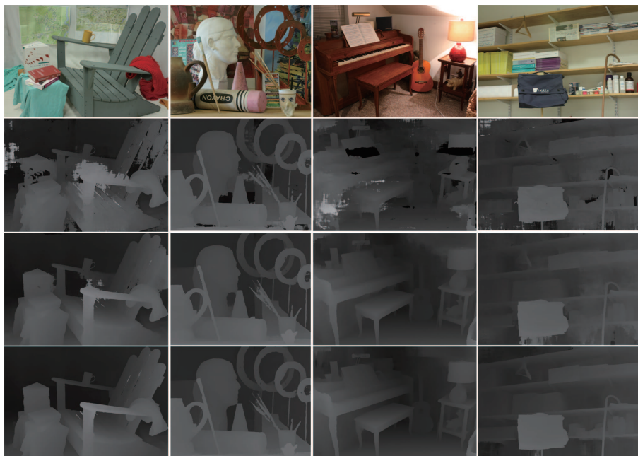
Figure 5 (Color online) Disparity maps achieved by PSMNet. The 1st row shows the color images in the training set of Middlebury 2014, the 2nd row shows the results of PSMNet-A, the 3rd row shows the results of PSMNet-C, and the last row shows the results of PSMNet-E.
