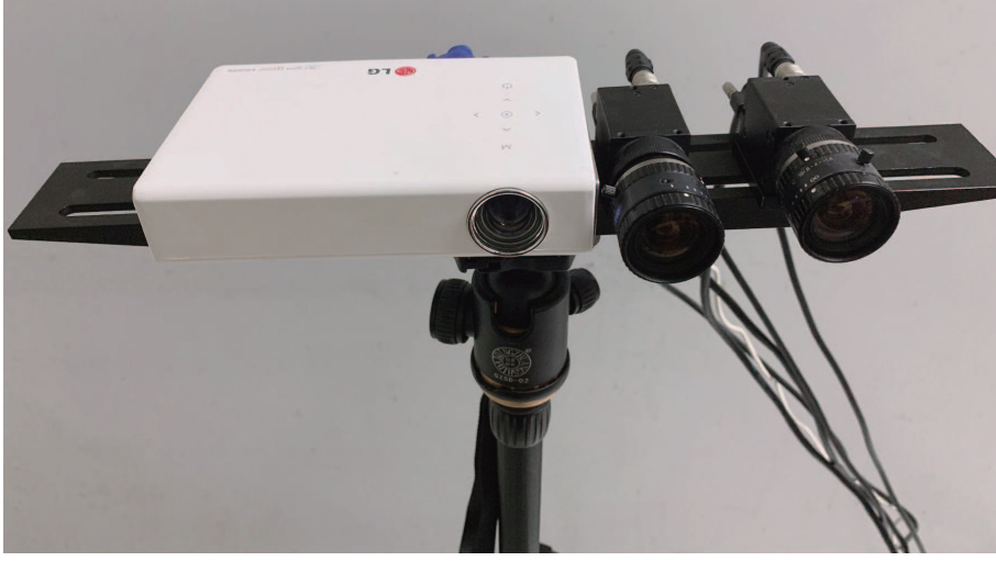
Figure 1 (Color online) An illustration of the structured light system.
