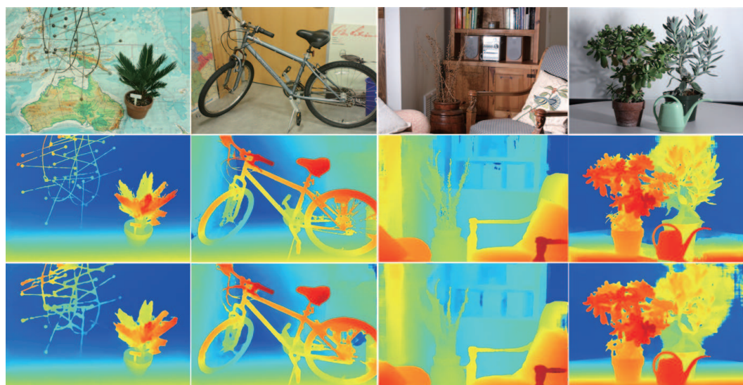
Figure 6 (Color online) Disparity maps achieved by PSMNet-E on the test set of Middlebury 2014. The 1st row shows the color images in the test set of Middlebury 2014, the 2nd row shows the results of PSMNet-E, and the 3rd row shows the results of PSMNet model in [9].
